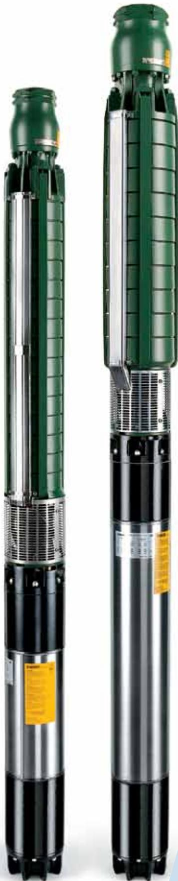
Borehole electric 8" and 10" radial pumps able to reach high heads. Thanks to the limited axial dimensions of the wet-end these machines feature a high number of stages with limited length so as to make them compact and reliable. Very solid machines, designed to last and to always ensure peak performance and efficiency under harsh conditions of use at great depths of installation and extremely high heads.
