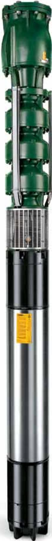
Borehole electric pumps coupled with asynchronous submersible motors at 2.900 and 1.450 rpm. Tried and tested machines whose ideal use is for lifting medium flows and medium heads. These pumps are installed in wells all over the world with unanimous satisfaction of the users. Sturdy construction of cast iron, bronze or stainless steel with impellers locked on the stainless steel shaft. Their design makes them especially suited for lifting water containing sand.
